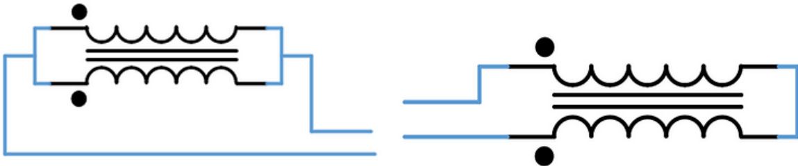
Left: common-mode measurement. Right: Differential-mode measurement.
